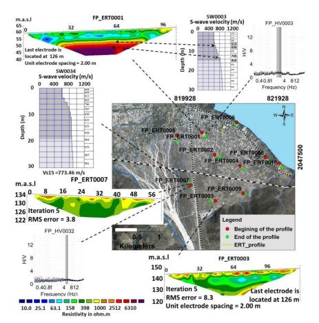
**Figure 13.** Comparison between ERT and MASW results for measurements completed on the central and upper parts of the alluvial fan.
