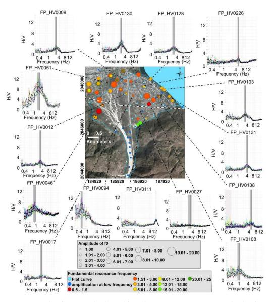
**Figure 7.** Examples of HVSR results obtained for ambient noise measurements completed on/near the alluvial fan. Circles on the central map indicate the resonance frequency, f0 (color), and amplitude of the f0 peak (size of circle).
