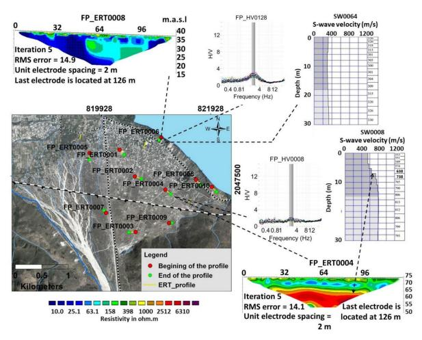
Figure 14. Comparison between ERT and MASW results for measurements completed on the lower part of the alluvial fan, near Lake Azuei.
