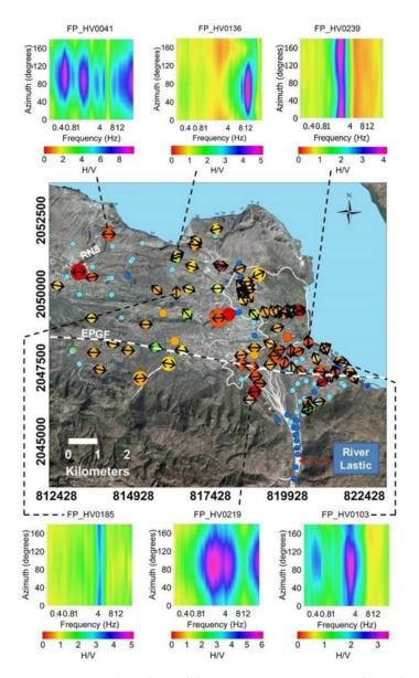
**Figure 8.** Azimuth analysis of the HVSR measurements performed in Fond Parisien. Graphs on top and at the bottom show the amplitude distribution over frequency and azimuth for six measurements. The double arrow on top of the f0-amplitude circles (see legend in the previous Figure 7) represents the preferential shaking orientation (of ambient noise).
