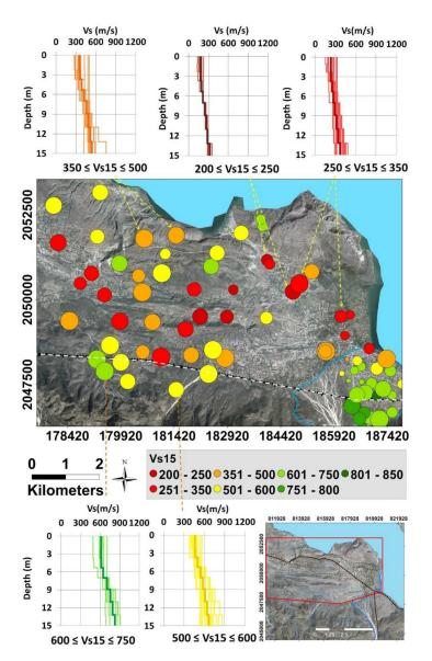
**Figure 6.** Vs profiles determined for the central and western part of Fond Parisien (down to a depth of 15 m). Vs15 values are represented in the central map by colors for each investigated site. See also the approximate location of the EPG Fault.
