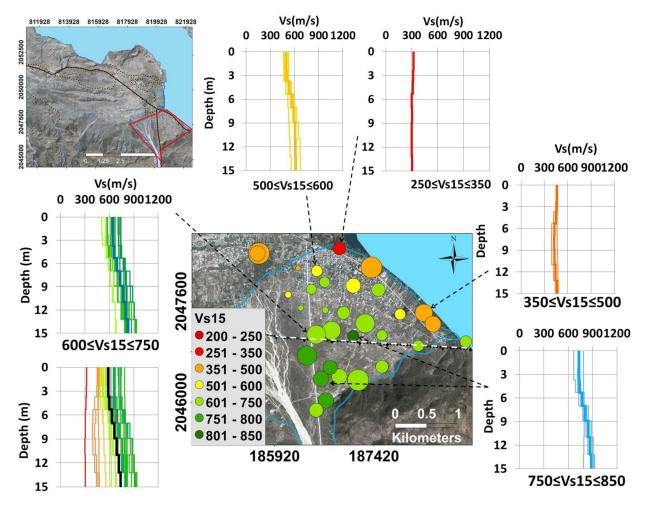
**Figure 5.** Vs profiles determined for the village "La Source" and the alluvial fan (down to a depth of 15 m). All profiles in this area are summarized in the lower left corner with an average Vs log of this area outlined in black. Average Vs15 values are represented in the central map by colors for each investigated site. See also the approximate location of the EPG Fault.
