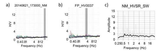
**Figure 10.** (a) HVSR curves from the Tromino single station measurements completed near the NM site; (b) HVSR results for the ambient noise recorded by the NM station; (c) HVSR curves computed from S-wave windows of earthquake recordings.
