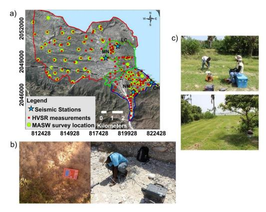
**Figure 3.** (a) Location of the HVSR measurements (red points), seismic stations (blue stars) and seismic profiles (for Multichannel Analysis of Surface Waves (MASW), analysis, light green circles) in Fond Parisien, with outline of EPGF (middle part of the map). (b) Photographs of ambient noise TROMINO (left) and CityShark recorders (right, with Lennartz 1Hz seismometer) and installation. (c) Photographs of seismic profile and seismic source (hammer impact).
