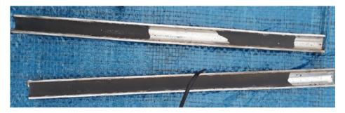
Figure 3. PbS scales deposited in tubes from the test heat exchanger.
