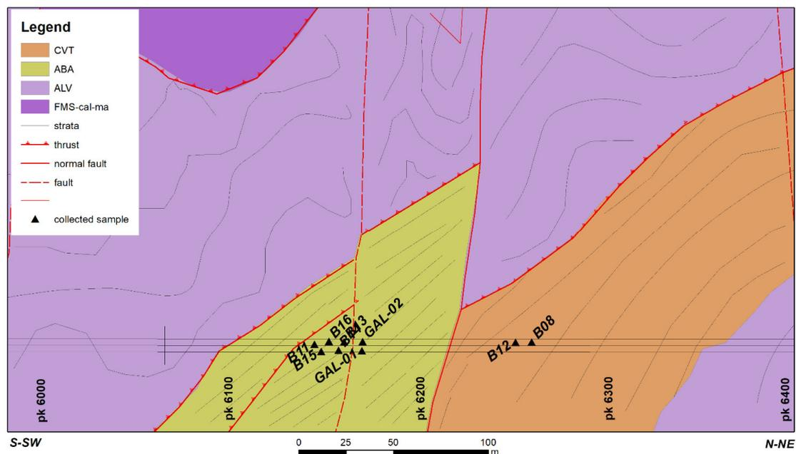
**Figure 9.** Location of sample collected along tunnel section from 6100 m to 6300 m chainage (pk). Geological unit codes: ALV, Argille Varicolori Superiori Fm.; ABA, Albanella/Corleto unit; CBI, bio-litoclastic rudist limestone fm.; CVT, Castelvete Formation; FMS, Monte S. Arcangelo Fm. with calcareous-marly lithofacies (FMS-cal-ma).
