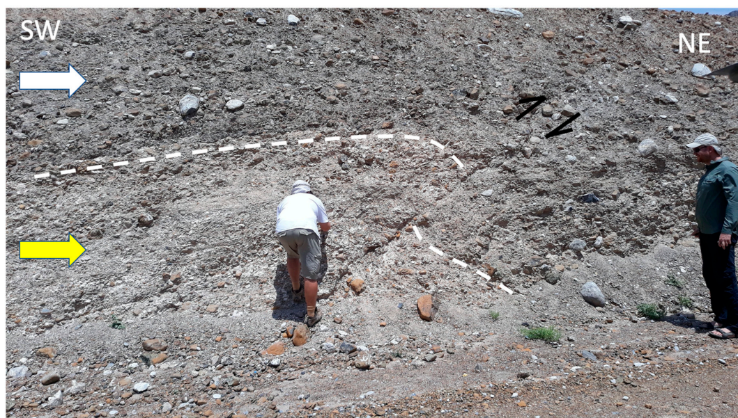
Figure 4. Upper unconsolidated samples (white arrow), and lower consolidated layer (yellow arrow) in fault 6. The displacement is ~1 m. Note the erosional contact between the two conglomerates (white dashed line). Also note drag folding!
