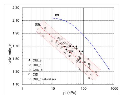
Figure 9. Steady state conditions of the specimens of Cervinara ash in the compression plane.
