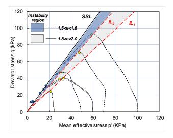
Figure 5. Instability lines and instability regions of specimens with different void ratios.
