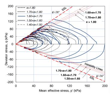
Figure 8. Stress paths in compression and extension tests.
