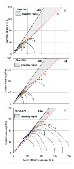
**Figure 6.** Stress paths of triaxial compression tests on anisotropically consolidated specimens (CAU\_c) and CIU\_c tests having void ratios ranging between: (**a**) 1.8–2.0; (**b**) 1.7–1.8; (**c**) 1.6–1.7.
