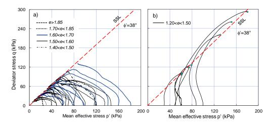
**Figure 4.** Results of triaxial compression tests on isotropically consolidated specimens (CIU\_c tests) on reconstituted specimens of Cervinara ash: (**a**) brittle response; (**b**) ductile response.
