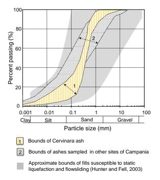
Figure 2. The grain size of eight different deposits of air-fall volcanic ashes in Campania.
