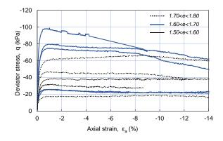
Figure 7. Stress-strain curves in extension tests (CIU\_e).
