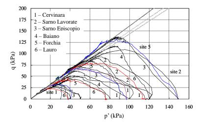
**Figure 3.** Results of undrained triaxial compression tests on undisturbed specimens of saturated air-fall volcanic ashes from six different sites in Campania.
