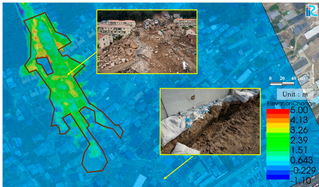
Figure 14. Horizontal distribution of the land deformation thickness in the residential area obtained by the numerical analysis. The brown line indicates the region where large rocks and driftwoods are inundated.
