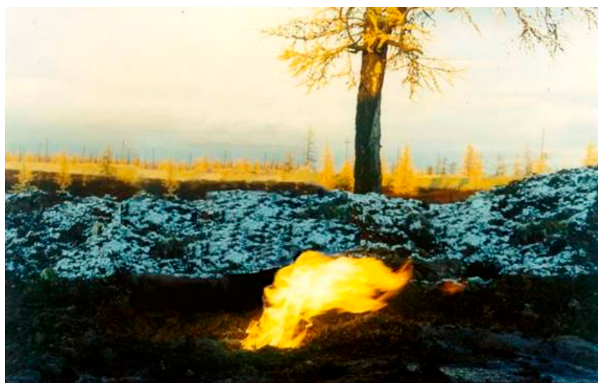
Figure 7. Burning of intrapermafrost gas rising from a depth of 15 m at the head of a geotechnical borehole (Zapolyarny field). Photograph by people from Fundamentproekt Company (number on the map: 13) [89].
