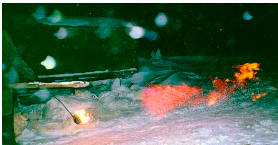
Figure 9. Release of intrapermafrost gas from a depth of 64 m in a test borehole. Bovanenkovo field. Photograph by Kondakov (number on the map: 19).
