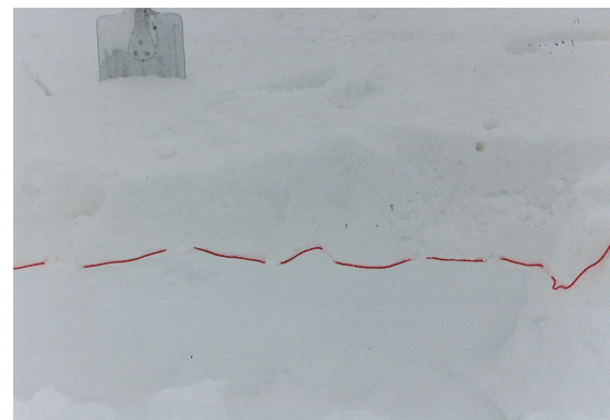
Figure A6. Left: A snow clod sintered to the deposit surface. Right: Trench through the snow cover on the plateau north-west of the cabins at Grand Moilles. The red rope shows the interface between the undisturbed snow cover and the deposits. The width of the spade is approx. 20 cm.
