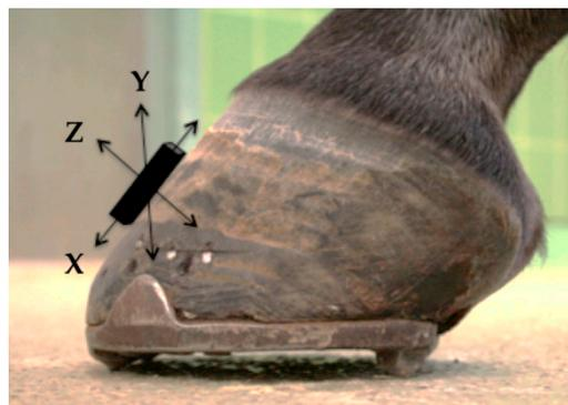
**Figure 2.** Schematic depiction of the accelerometer location on the dorsal hoof wall with the axes measured:  $x$ -axis proximodistal,  $y$ -axis mediolateral, and  $z$ -axis dorsopalmar/dorsoplantar.
