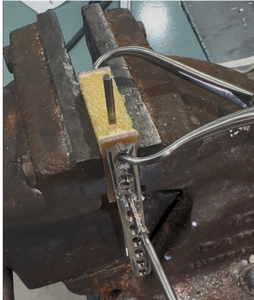
Figure 5. Benchtop replication of the failure mode. A block of fibre-filled, epoxy-laminated, 5 PCF open-cell rigid polyurethane foam (Sawbones® Pacific Research Laboratories, Vachon, WA, USA) was held in a table vice. The laminated surfaces formed the lateral and medial cortex. A 4 mm Steinmann pin was inserted in a proximodistal orientation, within the open-cell foam, replicating the clinical scenario of an intramedullary rod in metaphyseal bone. A 3.5 mm LCP was applied, with screws in a mediolateral trajectory. Contact between the rotating drill bit and the screw during plate application resulted in linear motion of the pin.
