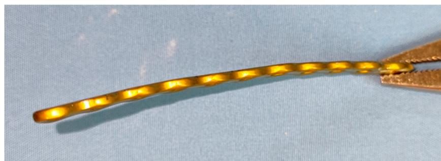
**Figure 5.** Pre-contoured 90 mm-long 2.4/2.7 locking plate.
