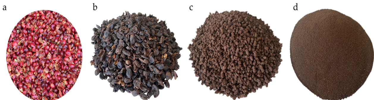
Figure 2. (a) Fresh coffee pulp, (b) dehydrated coffee pulp, (c) extruded coffee pulp, and (d) extruded coffee pulp flour (ECFP).
