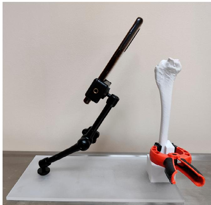
**Figure 2.** Self-made bone-holding device.
