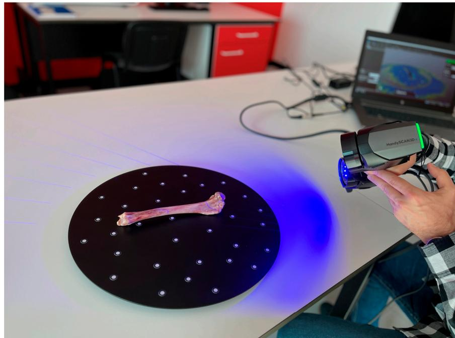
**Figure 1.** The digitizing process of the right canine tibia with intact menisci.
