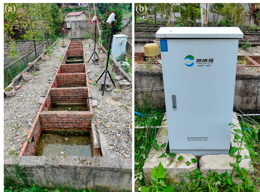
Figure 1. Simulated natural breeding pool (a) and water quality monitoring system (b). These red circles are camera locations.
