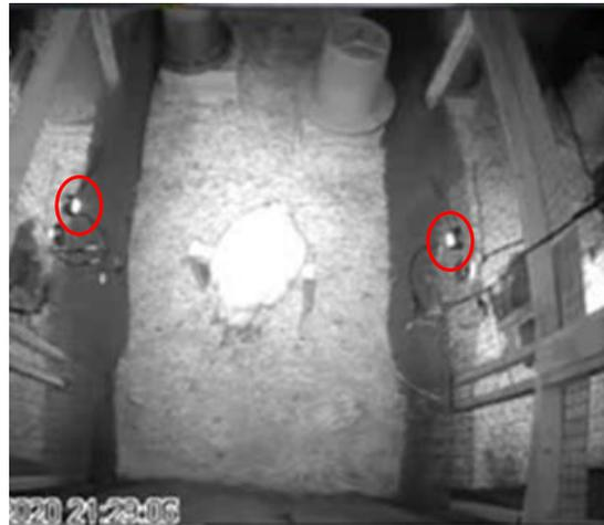
**Figure 2.** Camera framing displaying an overhead view of the pen with the bird perching for recording during lights-off. The positioning of cameras on either side of the perch is indicated in red.
