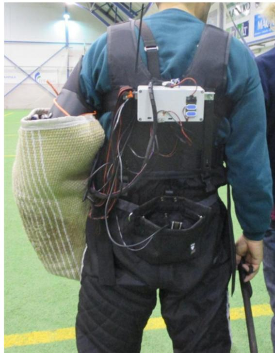
**Figure 2.** Measurement equipment on the helper.
