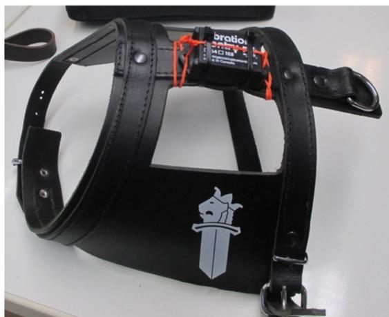
**Figure 3.** Three-dimensional accelerometer attached to dogs' harnesses.
