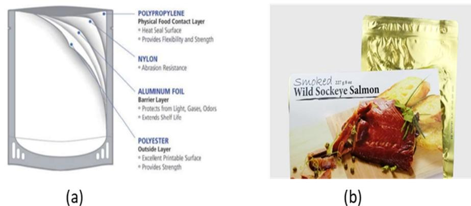
**Figure 4.** (a) Retort pouch structural construction (image courtesy: flairpackaging.com), (b) commercial retort pouch packaging for smoked salmon.
