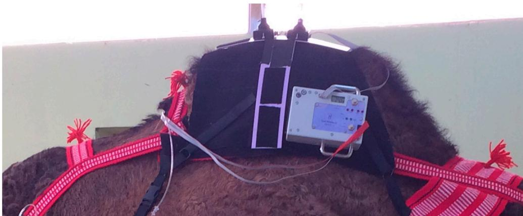
**Figure 4.** Cuboid thermal unit mounted on a camel's hump.
