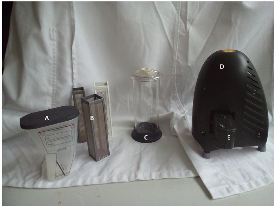
**Figure 1.** The supplied FECPAK<sup>G2</sup> equipment. A: Sedimentor; B: 1 mm white pre-filter and 600 and 425  $\mu\text{m}$  silver filters; C: filter cylinder; D: Micro-I imaging device; E: FECPAK<sup>G2</sup> cassette, inserted into Micro-I.
