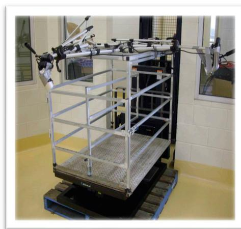
**Figure 1.** Platform and crate used to expose sheep to simulated ship movement.
