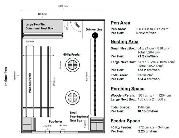
**Figure 2.** The layout and dimensions of one indoor pen at the layer facility showing the placement and dimensions of all resources. The resource allocation per hen is also indicated. Each pen was of the same set-up except three of the nine pens (balanced across treatments), contained a radio-frequency identification component box that one of the small nest boxes was placed upon.
