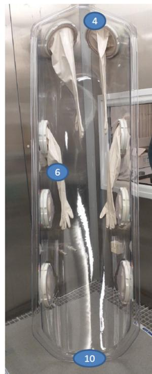
**Figure 4.** EpiShuttle hardtop showing the numbered challenge test locations (4,6 = MS2 on coupons; 10 = MS2 in organic liquid).
