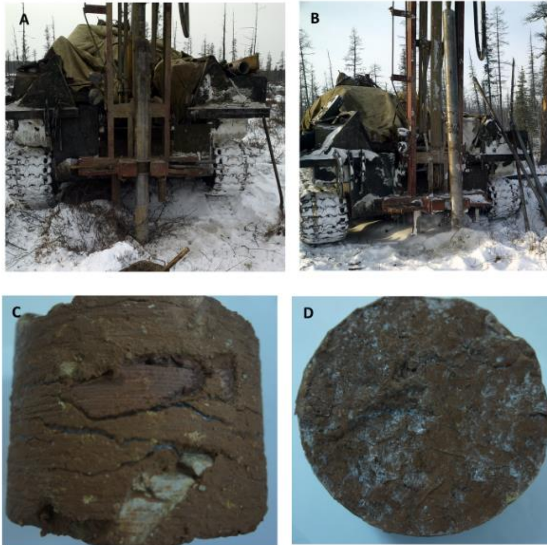
Supplementary Figure 1. Illustration of the permafrost collection process. A and B : core drill. C and D: permafrost specimen following shipment.
