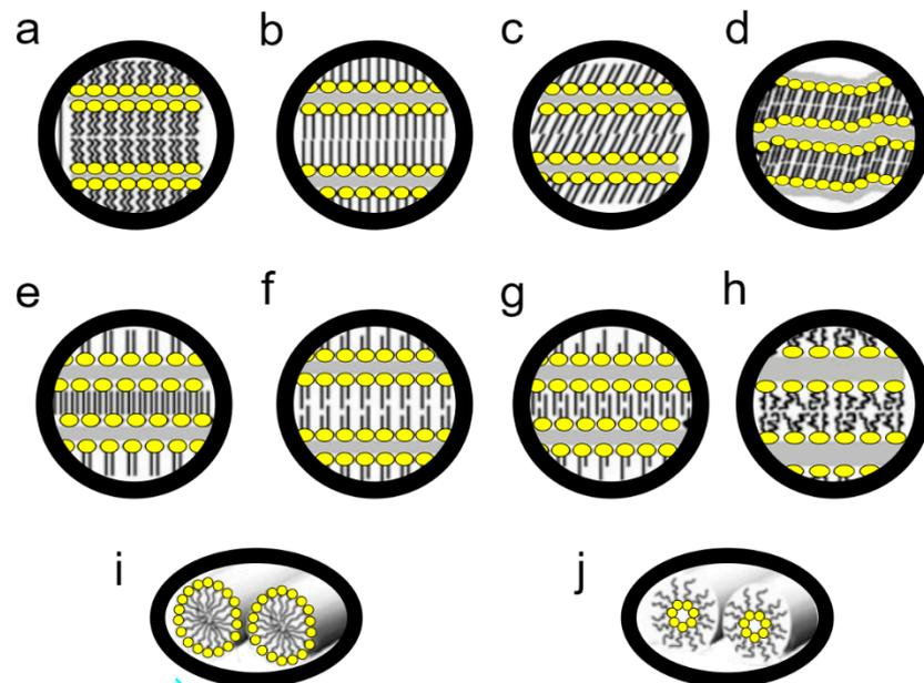
**Figure 4.** Selected lipid phases. (1) lamellar: (a) crystalline,  $L_c$ ; (b,c) gel  $L_{\beta}$  differing in the tilt of the chain types; (d) rippled gel  $P_{\beta}$ ; (e–g) gel  $L_{\beta}$  with a varying interdigitation; (h) liquid crystal,  $L_{\alpha}$ . (2) hexagonal: (i)-regular,  $H_I$ ; (j)-inverted,  $H_{II}$  (data from [57], figure according to Koynova and Tenchov [57], adapted and redrawn).
