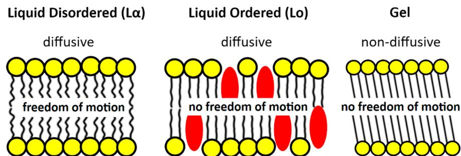
**Figure 3.** Structure and differences between the phases  $L_{\alpha}$  (disordered liquid crystal), the intermediate form  $L_o$  (liquid-ordered), and  $L_{\beta}$  (gel); red oval—hopanoids (data from [38,55]; elements of the figure by Faller [38] were used).
