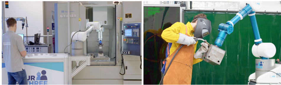
Figure 14. Two of the final prototypes at the end-user facilities; (left): Arm at the company STODT (The Netherlands) supporting a person during the loading and unloading of a machine; (right): Arm at the application scenario of the company WOLL (Germany) supporting a person during a welding task by holding and positioning of the workpiece (©FourByThree; permission granted).
