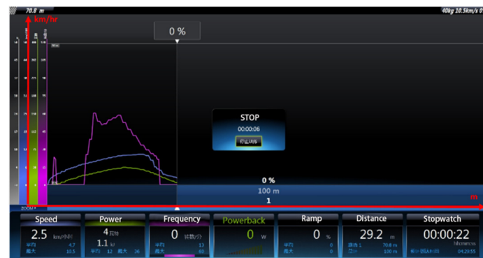
Figure 14. Results for flat road, cyclist weight 40 kg, and lower-arm three-phase short-circuit braking.
