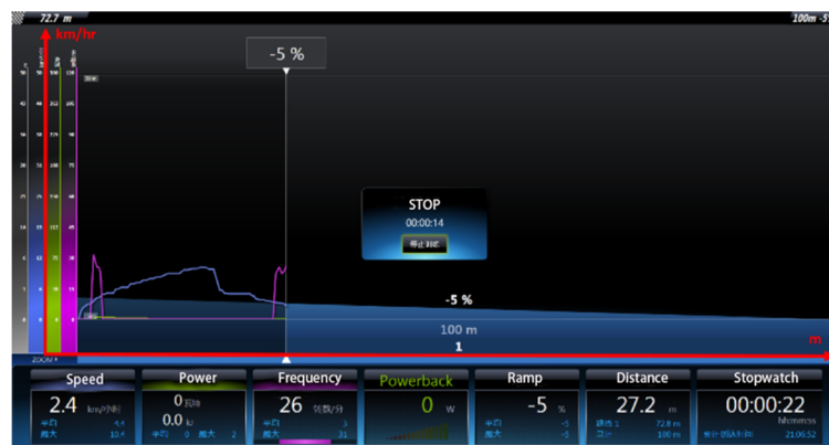
Figure 19. Results for road slope -5\% , cyclist weight 40 kg, and electromagnetic reversal braking.
