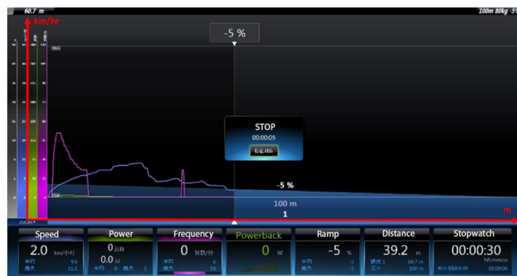
Figure 17. Road slope -5\% , cyclist weight 80 kg, and lower-arm three-phase short-circuit braking.
