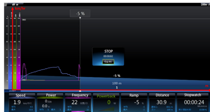
Figure 15. Results for road slope -5\% , cyclist weight 40 kg, and lower-arm three-phase short-circuit braking.
