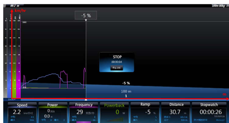
Figure 21. Results for road slope −5%, cyclist weight 80 kg, and electromagnetic reversal braking.
