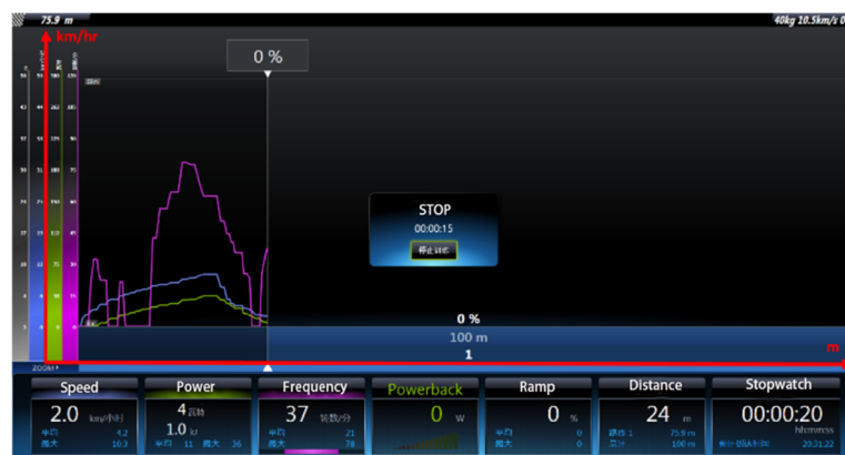
Figure 18. Results for flat road, cyclist weight 40 kg, and electromagnetic reversal braking.
