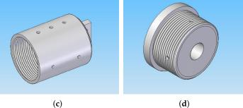
**Figure 15.** Gearbox 1:4 structure components. (**a**) Gear 1:4; (**b**) Gear unit pulleys; (**c**) Gear housing; (**d**) Gear cover.
