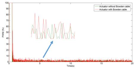
Figure 9. Actuator PWM signals with Bowden and without Bowden cable.
