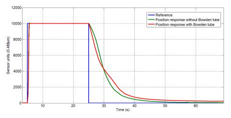
Figure 8. SMA actuator with Bowden cable vs. without Bowden cable (Figure 7 enlarged).
