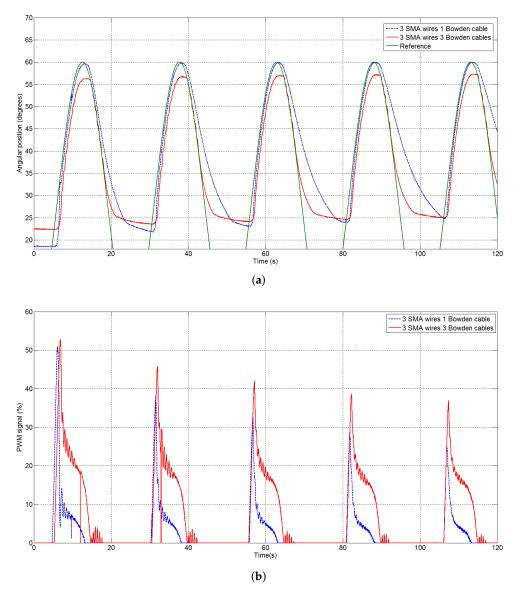
**Figure 11.** Multiple SMA wires actuator. (**a**) SMA based actuator position response, (**b**) PWM signals corresponding to SMA based actuator response.
