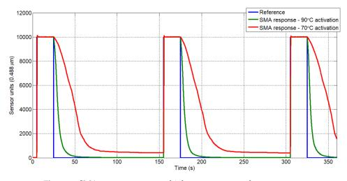
Figure 5. SMA actuator response: high temperature vs. low temperature.
