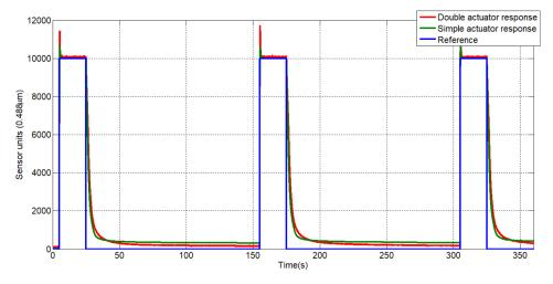
Figure 13. SMA double vs. simple actuators response.
