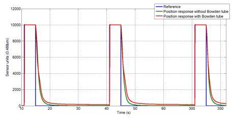
Figure 7. SMA of 0.51 mm diameter position response with Bowden cable vs. without Bowden cable.
