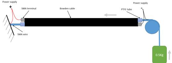
Figure 12. Double actuator configuration.
