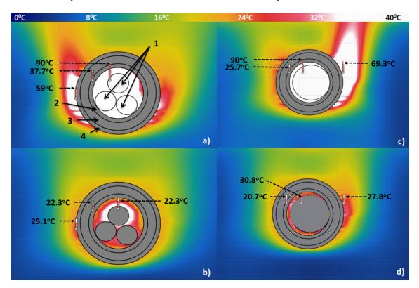
with three SMA wires has an approximately 0.3% strain and only one wire has approximately 0.1% strain, which implies that in the second case the heat is better dissipated.
