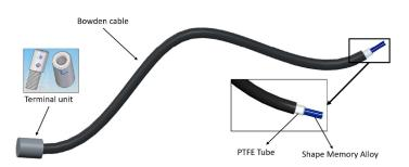
Figure 2. Flexible SMA-based actuator.
