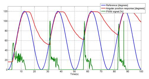
Figure 16. SMA-based actuator with gear 1:4 response.
