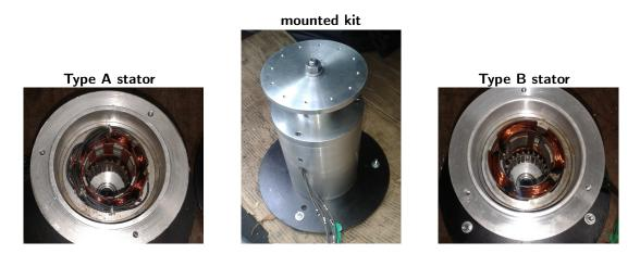
**Figure 9.** Top view of Prototypes A, on the left, and B, on the right; notice the eight "poles" in Type A and only four "poles" in Type B. A mounted kit is shown in the center, with a vertical rotor inserted in one of the carcasses. The perforated disk built in the upper position is used for mass unbalance tests.
