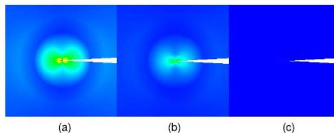
**Figure 8.** The Von Mises stress field around the crack tip with different applied voltages on piezoelectric patches: (a) 0 V, (b) 300 V and (c) 480 V [50].
