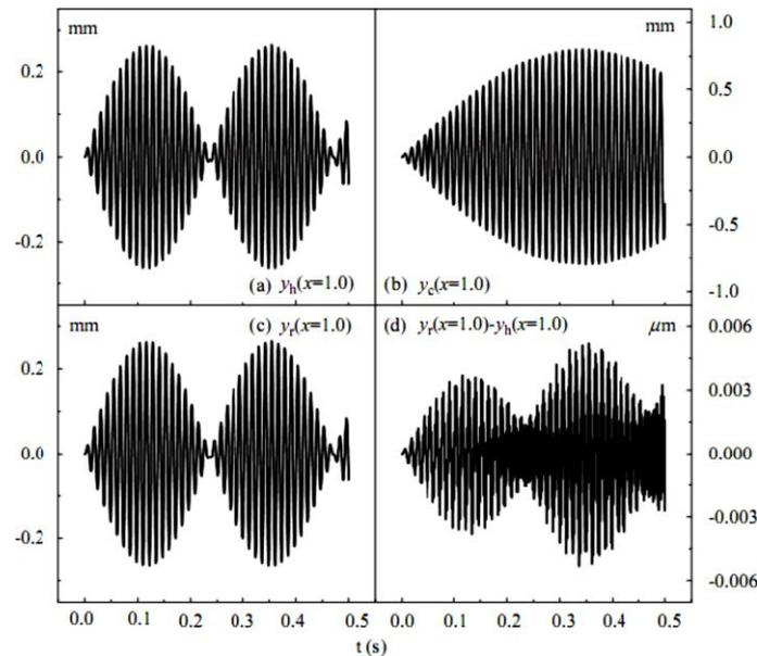
**Figure 4.** Time history of tip displacement predicted by proposed model for (a) healthy beam, (b) cracked beam, (c) repaired beam, and (d) difference between repaired and healthy beam [28].
