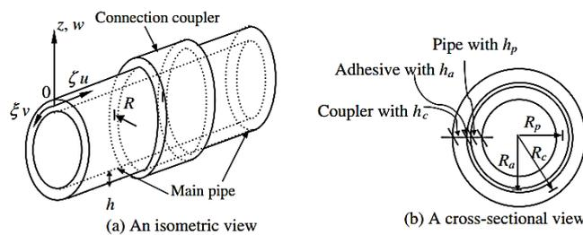
**Figure 11.** Schematic of adhesive joint with piezoelectric layer in coupler proposed by Cheng *et al.* [63].
