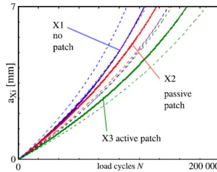
**Figure 6.** Summarized mean (—) and mean deviation (---) curves of crack length propagation  $a_{xi}$  versus load cycles  $N$  according to no applied patch for case X1 (top), applied passive patch for case X2 (middle) and applied active patch for case X3 (bottom). [35].
