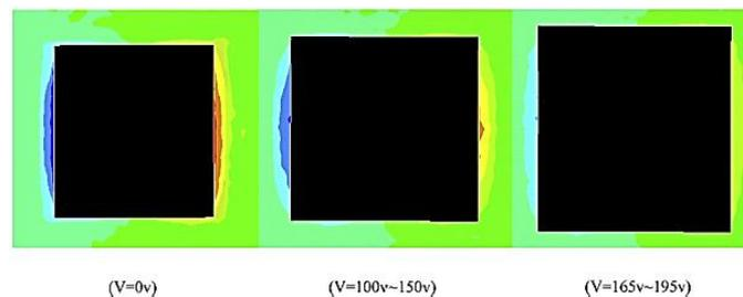
**Figure 9.** FEM simulation of shear stress distributions along delamination edges with different voltages ( $L_1 = L_2 = 0.1$  m,  $a = b = 0.1$  m,  $t = 0.005$  m) [52].
