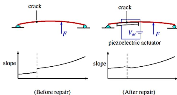
**Figure 3.** Slope continuity criterion for active repair [27].
