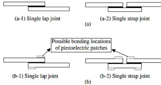
**Figure 10.** (a) Commonly used adhesive bonded joints; (b) the smart joints with piezoelectric patches bonded to them [57].
