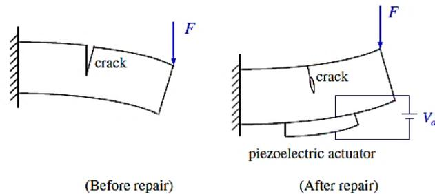
**Figure 5.** Fracture mechanics criterion for active repair [30].
