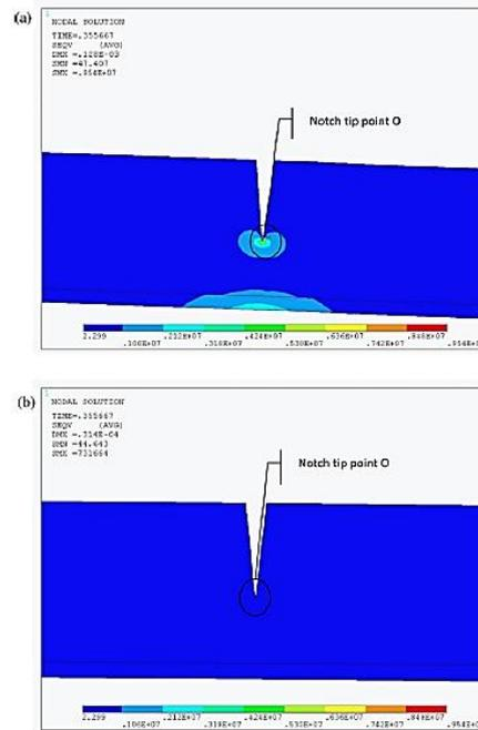
**Figure 7.** The Von Mises stress distribution at the notch position of the vibrating cantilever beam at (a) gain factor = 0 and (b) gain factor = 74 [37].
