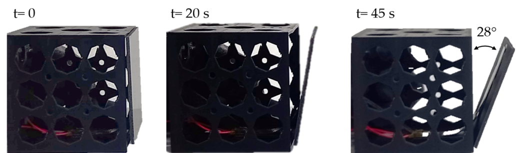
Figure 9. Opening of the top composite cover of a standard 1U polymeric CubeSat.
