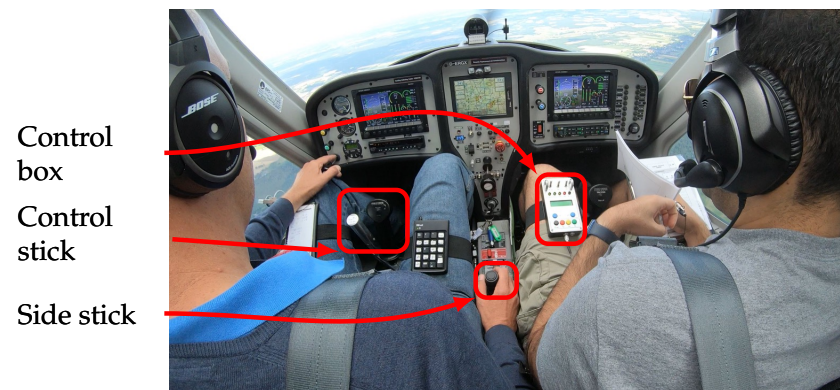
Figure 7. REMOS GX cockpit with flight test pilot (left) and flight test engineer (right) during flight.
