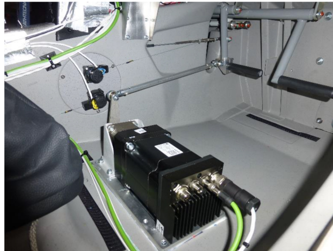
Figure 3. The rudder servo mounted inside the copilot's legroom, taken from [40].
