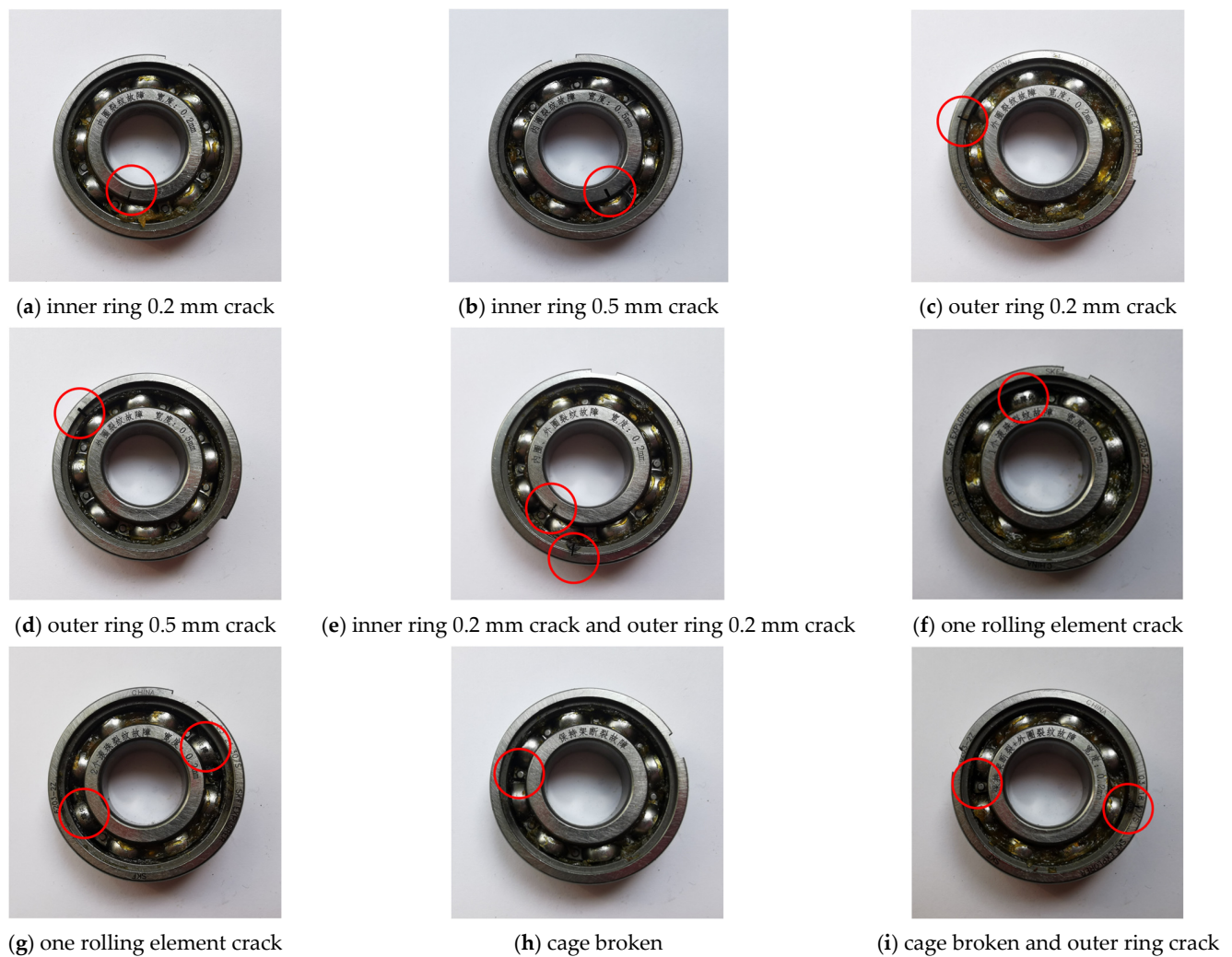
Figure 18. Bearing fault location diagram.
