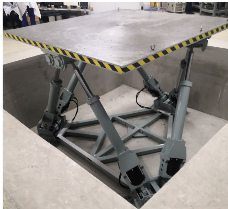
Figure 9. The experimental Stewart platform YBT6-2000.
