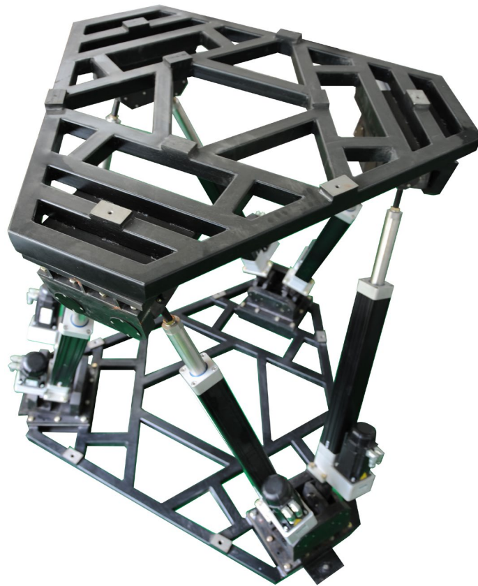
Figure 8. The experimental Stewart platform YBT6-250.
