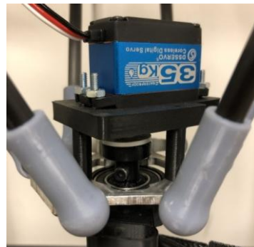
Figure 5. Servo motor-driven fourth axis for the end effector.
