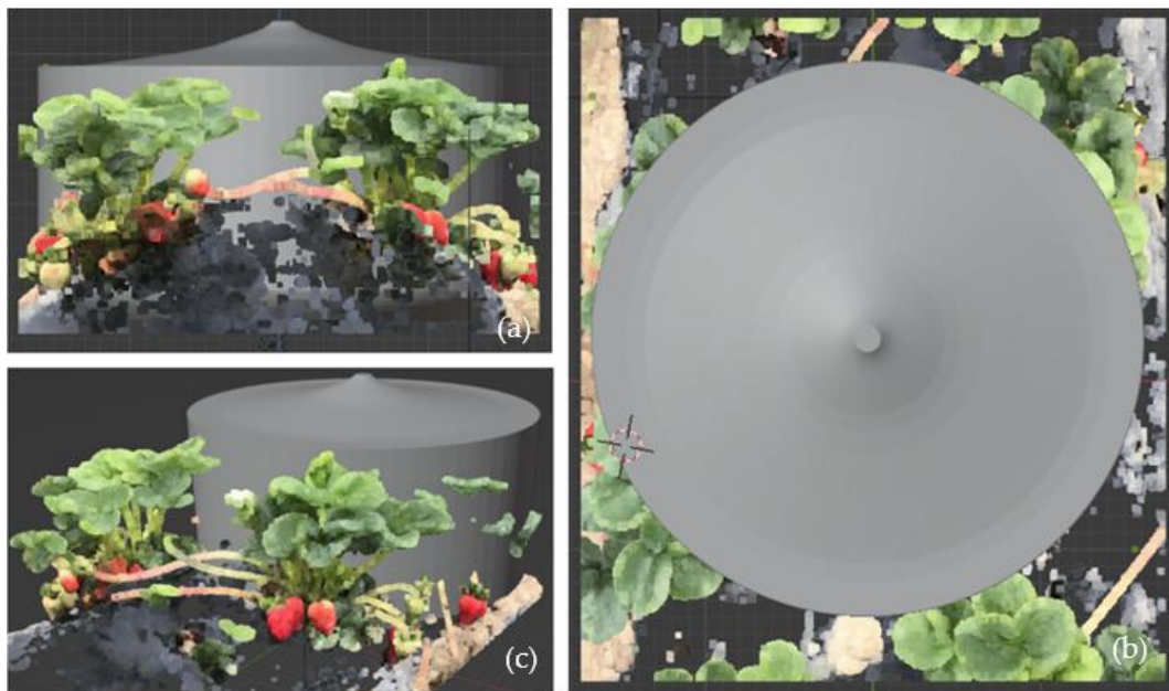
Figure 8. Simulated validation of the manually determined Delta X1 workspace compared to a typical two-plant-per-row strawberry field: (a) XZ planar view; (b) XY planar view; and (c) 3D view.
