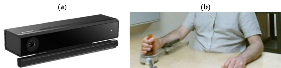
Figure 7. (a) Microsoft Kinect (K4W) v2. (b) A handheld end-effector with two degrees of freedom.
