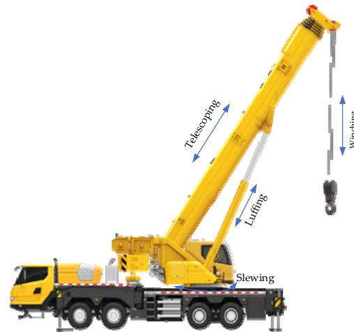
Figure 4. Schematic diagram of the truck crane working systems: luffing, slewing, telescoping, and winching systems.
