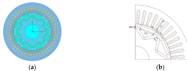
Figure 1. IPMSM model. (a) Structure of the IPMSM. (b) Schematic diagram of optimized parameters.
