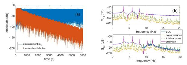
**Figure 7.** (a) The transient contribution. (b) The robust LPM used to obtain the noise/nonlinearity covariance and BLA.
