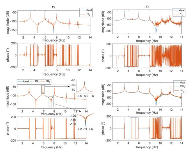
**Figure 12.** Conditioned and unconditioned FRFs in comparison to the correct linear estimate represented for selected states  $x_1$  and  $x_5$ .
