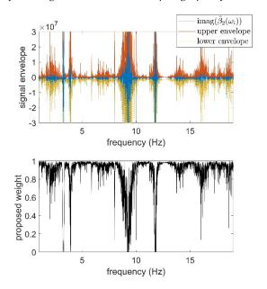
**Figure 11. Top**: The imaginary part of the estimated spectrum of the cubic term  $\beta_2$  and calculated envelopes. **Bottom**: The calculated weight based on Algorithm 2.
