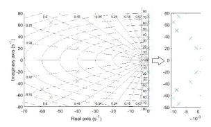
**Figure 8.** The poles of the simulation system  $(\times)$  in comparison to the poles of the steady-state Kalman state observer  $(\times)$ .
