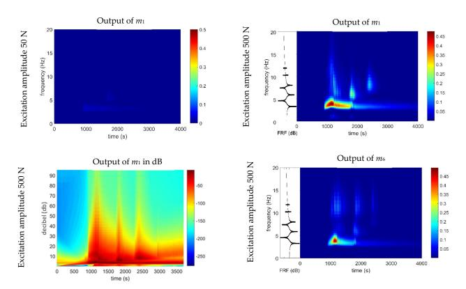
**Figure 3.** Wavelet-transformed output signal on a non-logarithmic scale, obtained for different values of excitation amplitudes measured at different mass positions.
