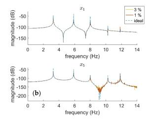
**Figure 13.** (a) The frequency content of the sampled colored noise acting on the measurement outputs. (b) The extracted FRFs under the prescribed measurement noise levels in Table 6.
