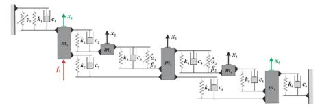
Figure 2. A substitute lumped mass discrete model with multi-degree-of-freedom.
