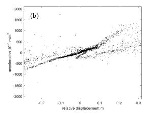
**Figure 5.** Corresponding side-view (acceleration vs. relative displacement) of the acceleration surface used for nonparametric modeling of nonlinearity at (**a**) mass  $m_1$  and the (**b**) junction between masses  $m_1$  and  $m_2$ .
