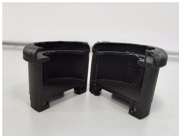
Figure 20. Element designed to keep the loads during the experiments carried out with weight. Source: authors.
