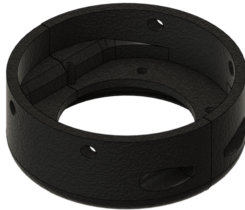
Figure 4. 3D-printed connection between segments. Source: authors.
