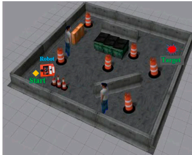
Figure 9. Path planning simulation environment for mobile robots in ROS-Gazebo.
