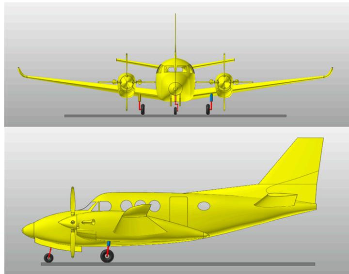
**Figure 8.** 7-DOF aircraft landing model based on RecurDyn.
