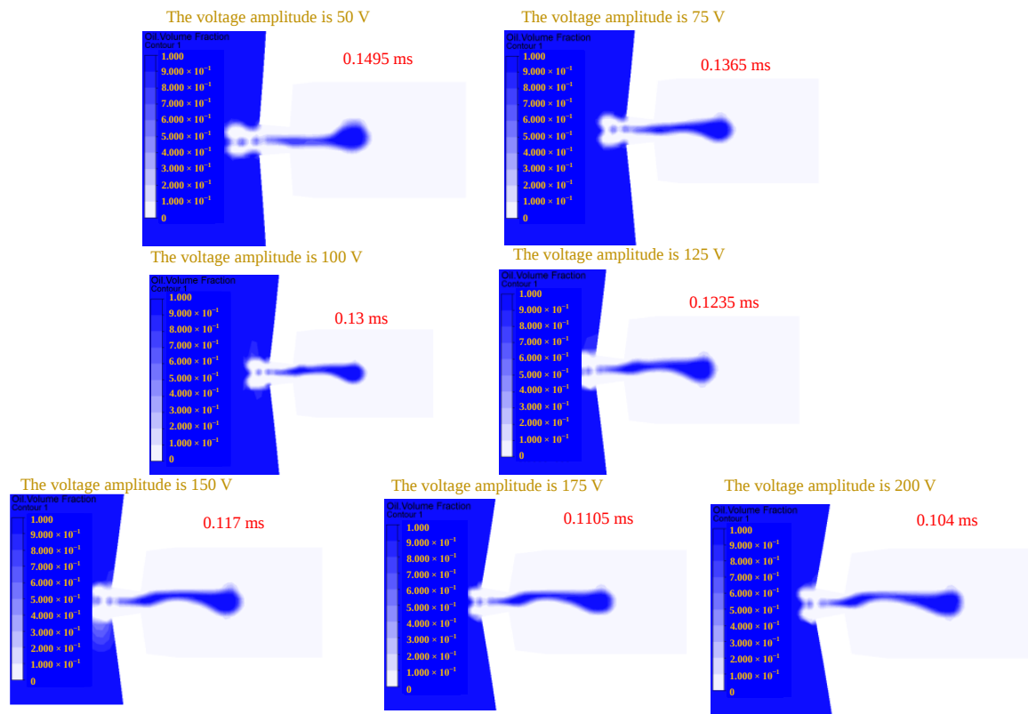
Figure 9. The change in droplet ejection state caused by the change in voltage amplitude.
