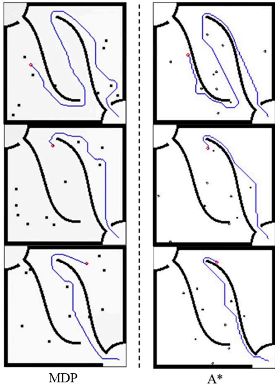
**Figure 7.** Comparison of MDP and A\* path planning in the case of 10 obstacles.
