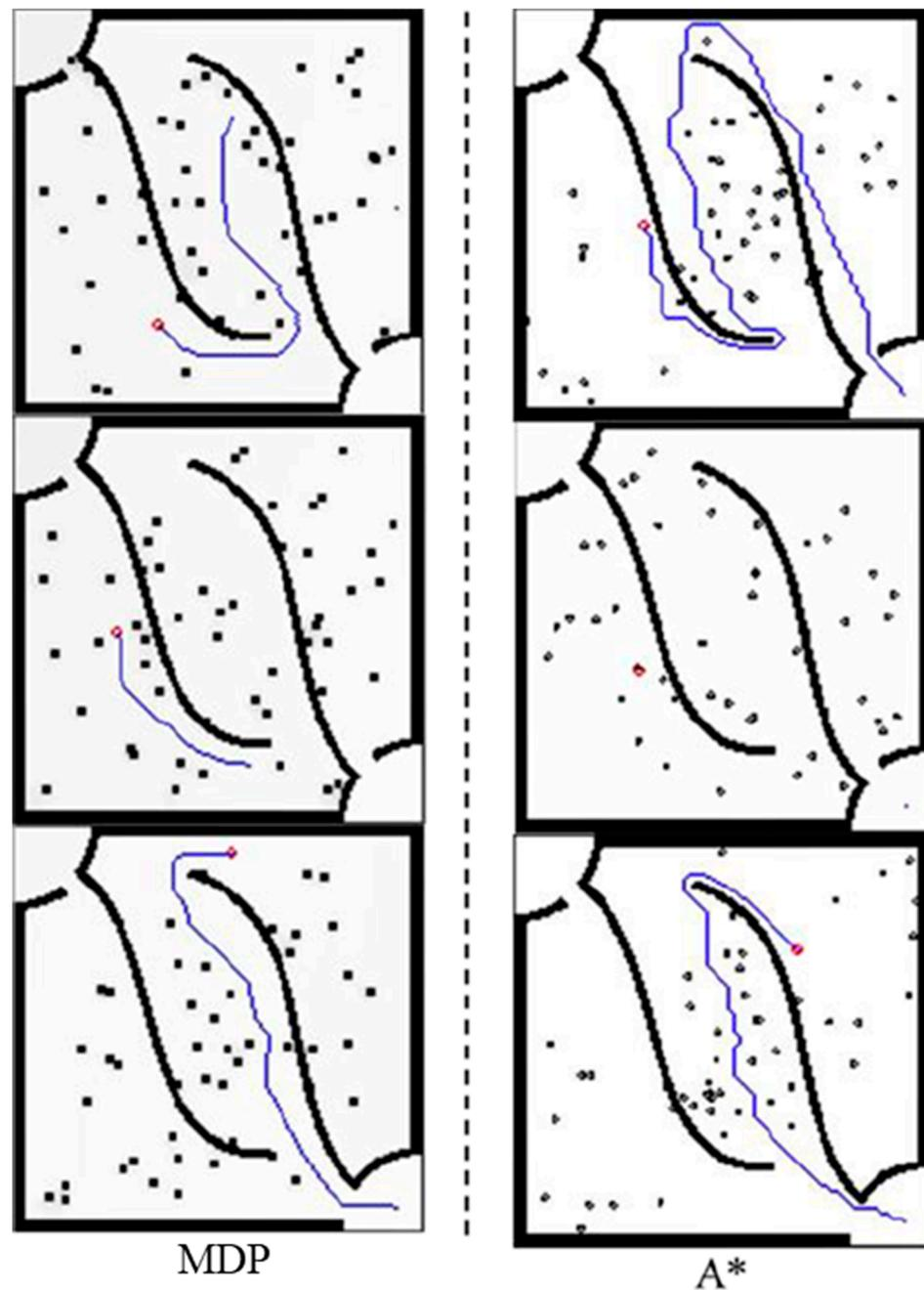
Figure 8. Comparison of MDP and A\* path planning in the case of 50 obstacles.
