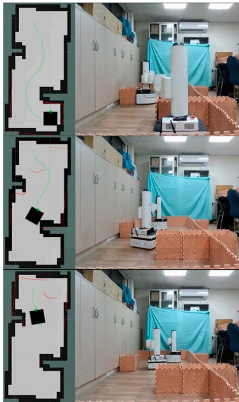
Figure 15. The path planning result in the environment with an unknown moving obstacle by the A\* algorithm.
