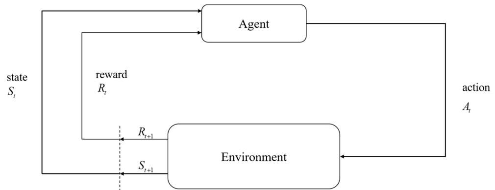
**Figure 1.** The interaction between the agent and the environment in the Markov decision process.
