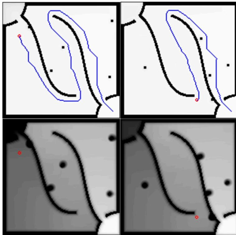
Figure 4. Real-time path planning with the distance cost to obstacles and walls.
