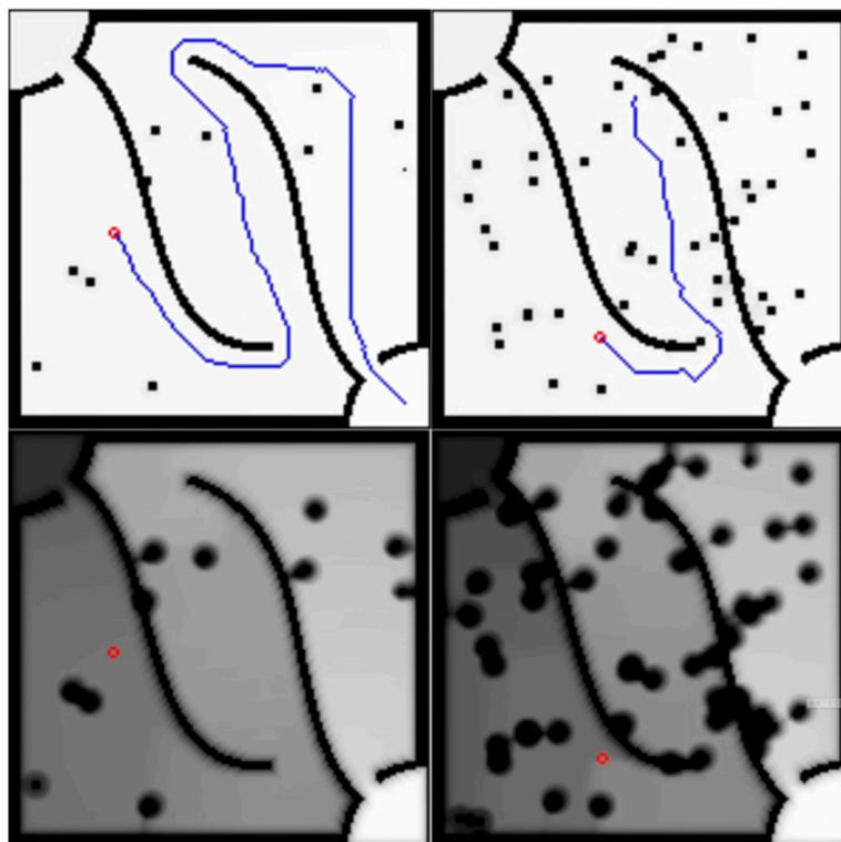
Figure 5. Real-time path planning with 10 and 50 obstacles.
