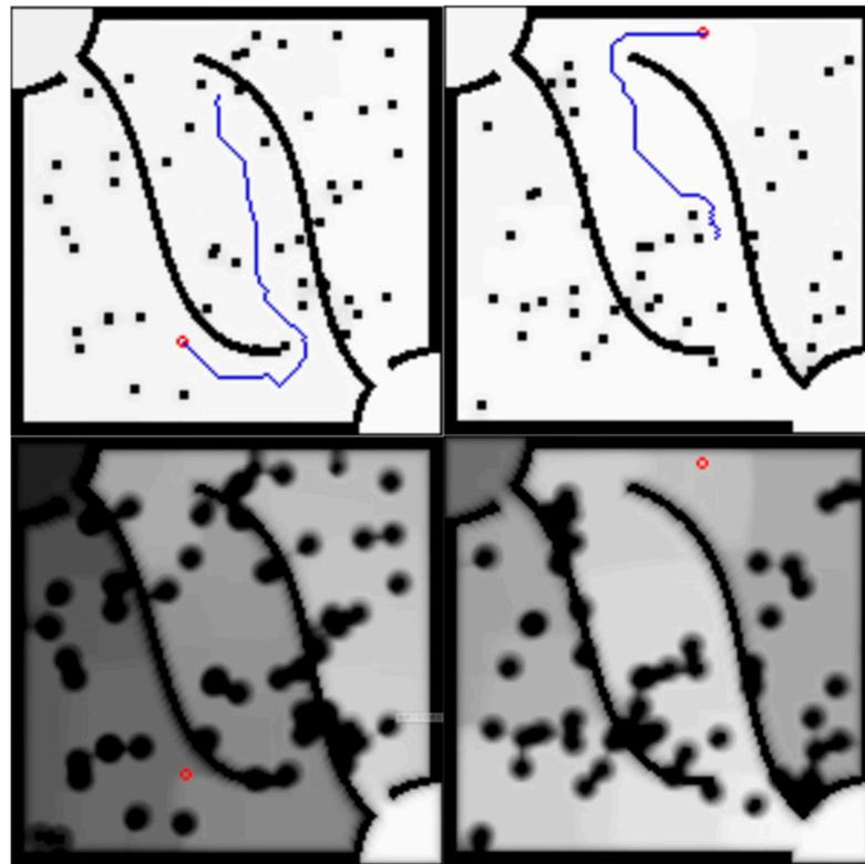
**Figure 6.** Real-time path planning with 50 obstacles on a changing map.
