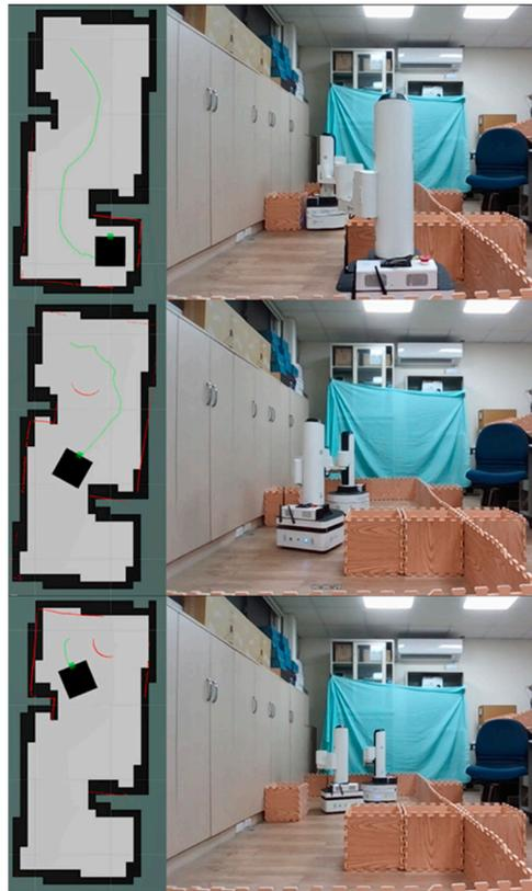
Figure 14. The path planning result in the environment with an unknown moving obstacle by MDP.
