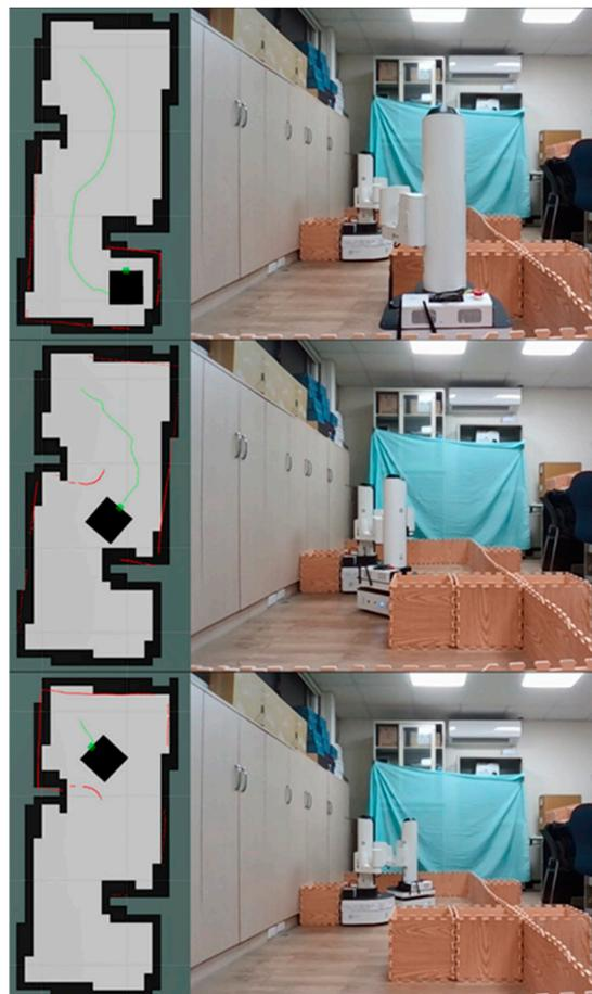
Figure 13. The path planning result in the environment with an unknown fixed obstacle.
