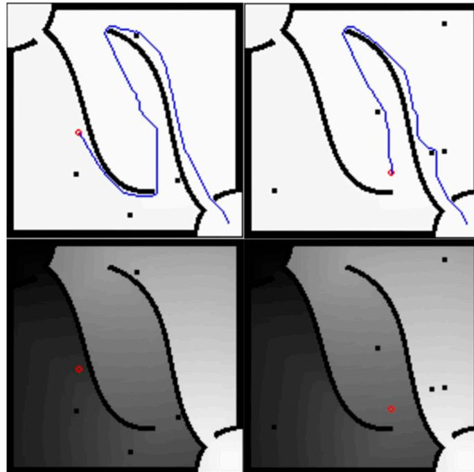
**Figure 3.** Real-time path planning without the distance cost to obstacles and walls.
