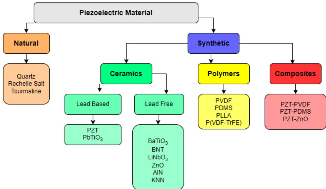
**Figure 4.** Classification of piezoelectric materials.
