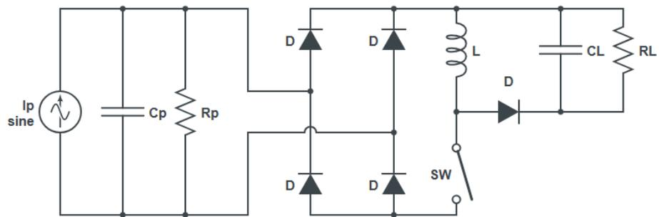
Figure 19. SECE energy harvesting circuit.
