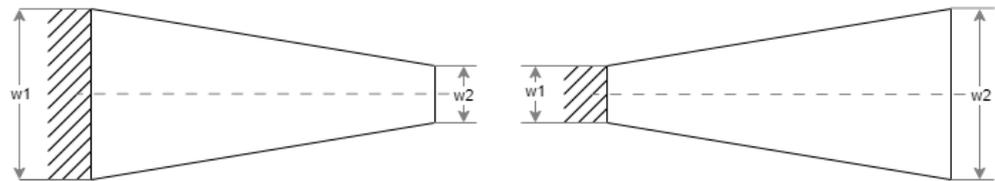
**Figure 7.** Direct and reverse trapezoidal cantilever.
