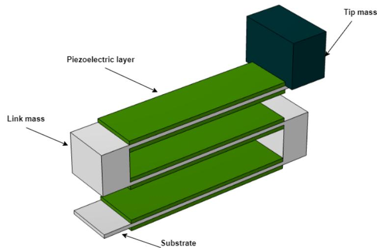
**Figure 10.** Schematic structure of fan-folded piezoelectric energy harvesters.
