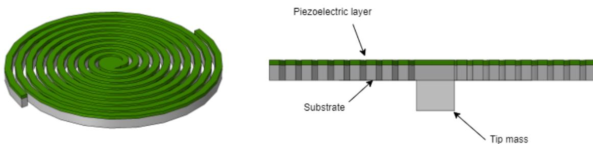
**Figure 11.** Schematic structure of spiral piezoelectric energy harvesters.
