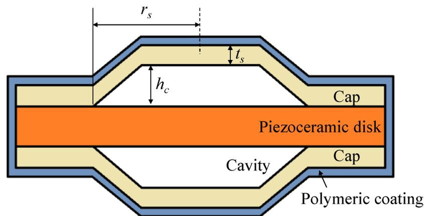
Figure 9. Schematic structure of piezoelectric cymbal transducer [182].
