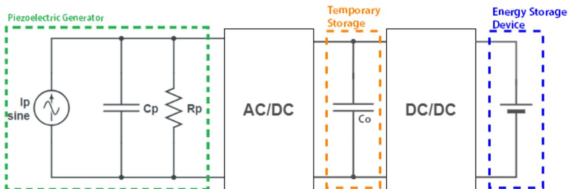
**Figure 16.** Generalized two-stage energy harvesting circuits.
