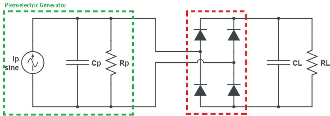
**Figure 15.** The standard full-bridge rectifier (FBR) circuit.
