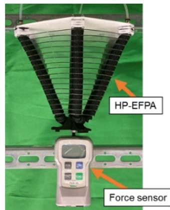
**Figure 12.** Experimental setup adopted for measuring pushing force.
