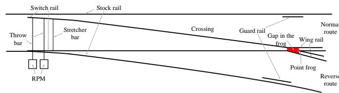
Figure 1. The schematic diagram for a simple turnout layout.
