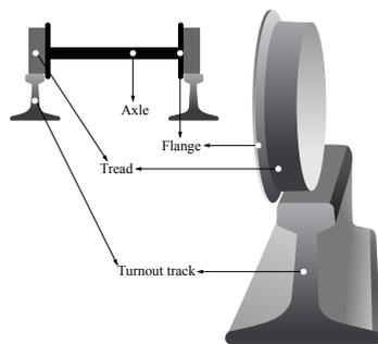
Figure 2. The schematic diagram for wheel–rail interaction.
