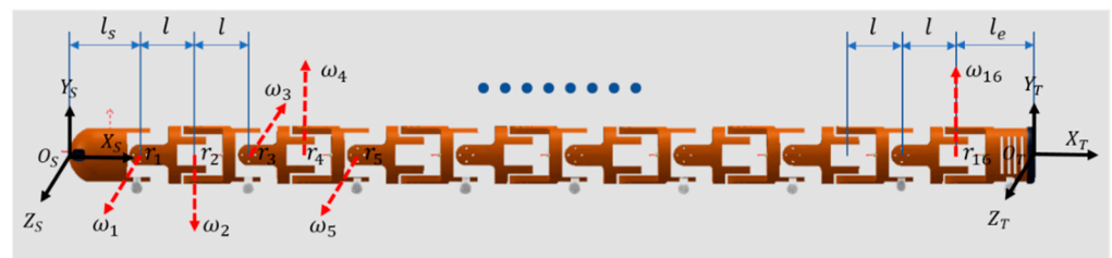
Figure 3. The screw coordinate model of snake robot.
