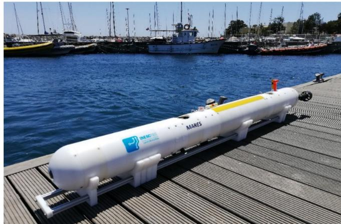
**Figure 1.** MARES AUV built using modular components.
