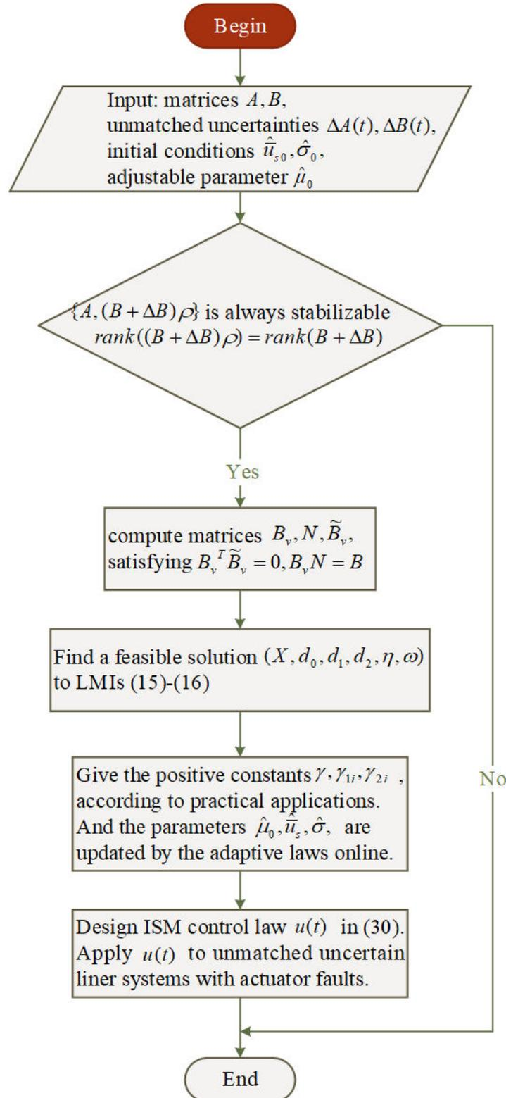
Figure 2. Flowchart of fault-tolerant control based on the ISMC algorithm.
