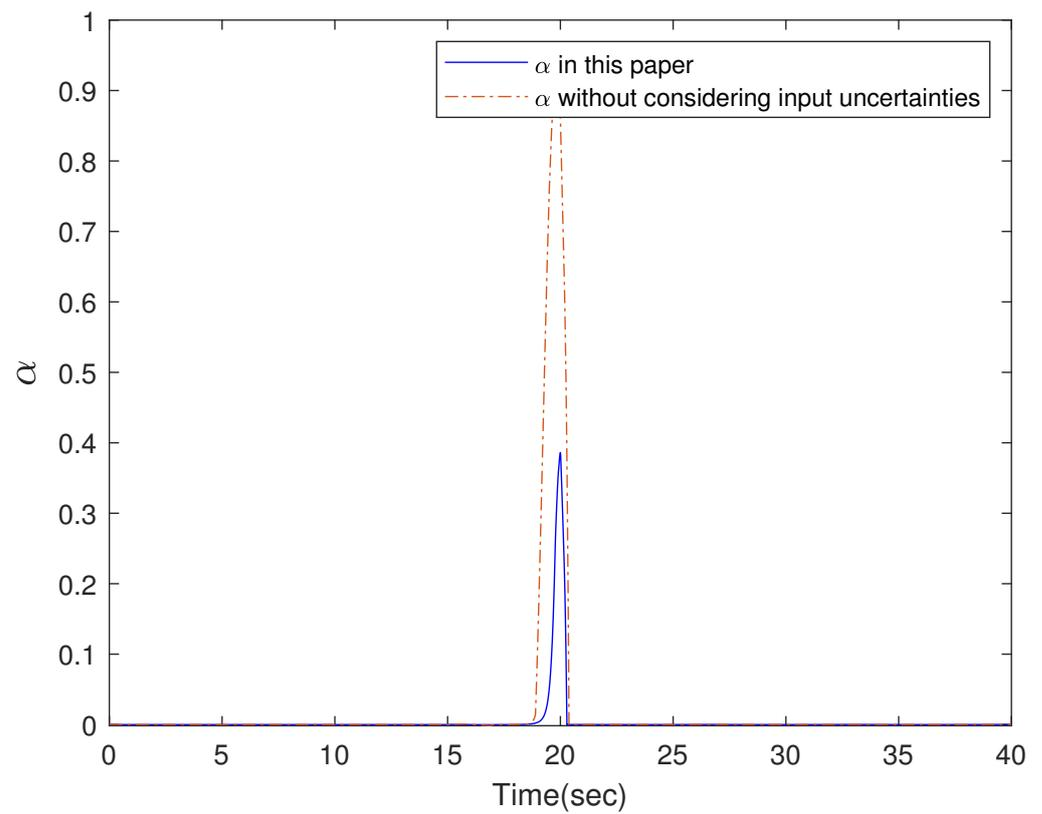
Figure 4. The comparison figure of the sliding surface response curves.
