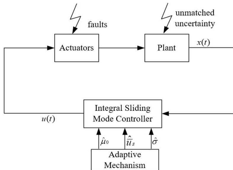
**Figure 1.** Structure diagram of ISMC fault-tolerant scheme.
