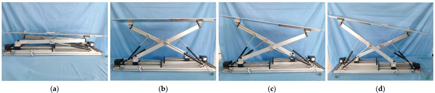
**Figure 16.** Different postures of the verification model: (a) Initial posture; (b) Lifting posture; (c) Right rotation posture; (d) Left rotation posture.
