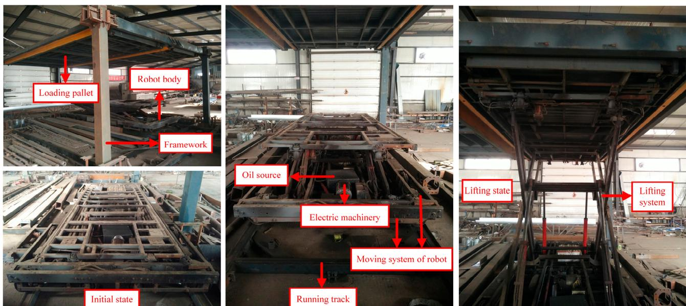
**Figure 18.** Experimental environment of the parallel lifting actuator on the stereo parking robot.
